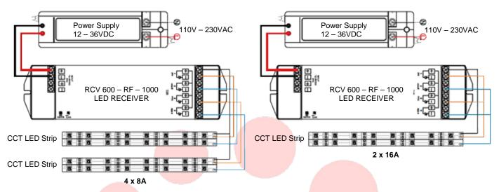
2) Receiver Connection Diagram for Multiple Units
